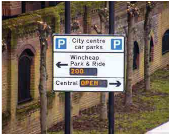
Figure 7.1 Real-time car park sign
